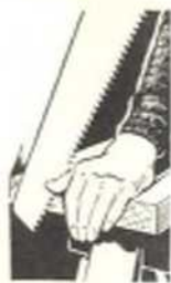
Starting the cut with a draw stroke
