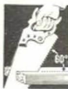
Proper angle for ripping
