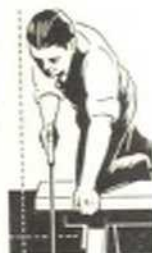
Proper position for cross-cutting
