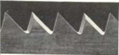
Shape of cross-cut saw teeth
