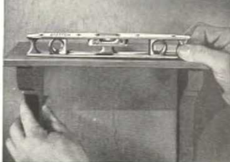
Leveling shelf with Disston A-10 Level
