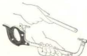
To insert blade in hack saw frame
