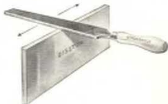
Draw-filing edge of cabinet scraper
