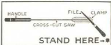
Second position for filing cross-cut saws
